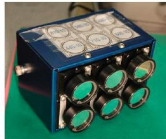
Multispectral camera array (MCA) imaging sensor
